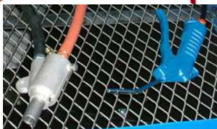
New blasting head with a flat entrance angle SP 500 P and blow gun SKB 610 AP optional
