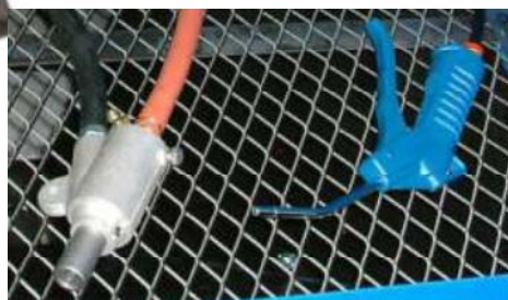
New blasting head with a flat entrance angle SP 500 P and blow gun SKB 610 AP optional
