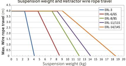
Suspension weight and Retractor wire rope travel
