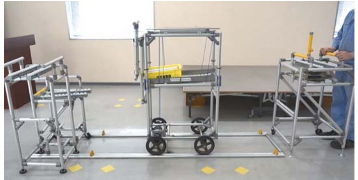
The cart has the mechanism which Zenmai motor is wound by adding the weight. The cart gets back automatically after remove the weight.
